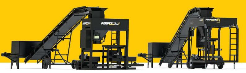
PERPETUAL® packaging concept begins with the transfer of materials prepared by a mixer onto a band. Materials delivered to the dispensing system via the band are transferred from here into bags. After the air is removed from the package, the movement of material in the system ends by pressing and closing the top of the bag. Since the pressing process is the main factor in the life of the packaged product, the pressing process will be ideal thanks to the four powerful pneumatic piston.
